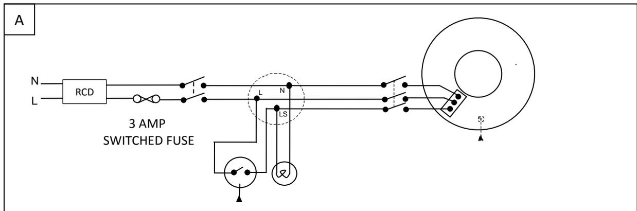
Wiring for control modules with no external switching
