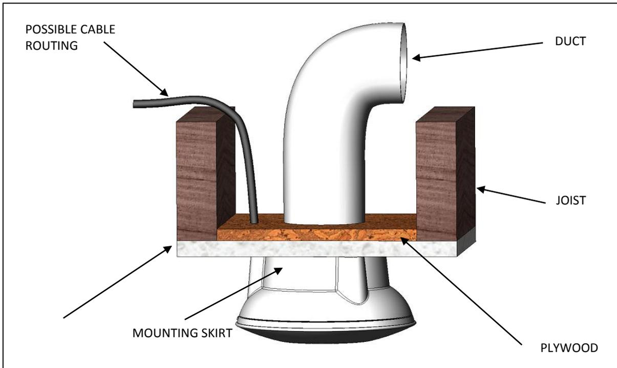
When surface mounting the iCON30, the mounting skirt should be used.
