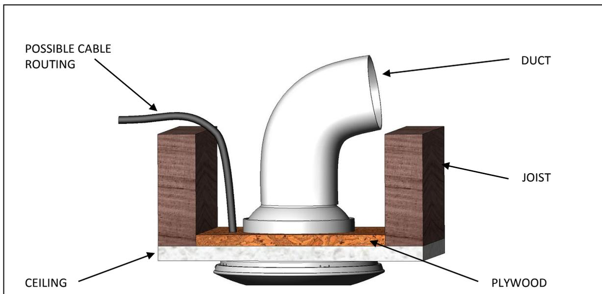
When recessing fans in the ceiling, a plywood support (min 18mm thick) should be mounted between the ceiling joists. Fans should not be fitted to unsupported plaster board.
