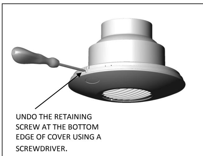
The front cover fan has a bayonet type fitting. To remove, undo the retaining screw at the bottom edge of the cover using a screwdriver, then rotate the cover a few degrees anticlockwise and remove. To refit, reverse the above procedure.
